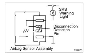
(3) Electrical Connection Check Mechanism
